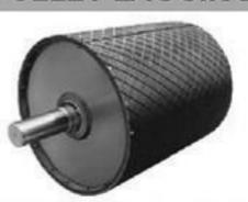
Pulley Lagging eliminates belt slippage. The diamond groove pattern splits the water and deflects it in to the grooves away from the pulley, hence increasing pulley life. Plain rubber pulley lagging also available.
