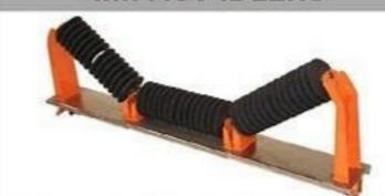
Impact Idlers protect the belt by absorbing impact at loading point. Generally they are 20° or 30° trough, however idlers with 45° or other troughing angles can also be utilized based on the application & inclination.
