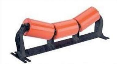
Generally available with side rollers inclined at 20° or 30°, idlers with 45° troughing angles or others, used for conveying Bulk Material.
