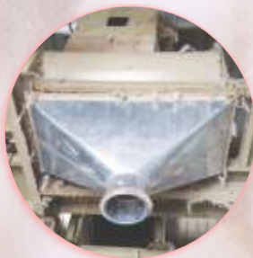
Separation of small size Stone, Sand and Kaudi by Application of Capsule Jali with G.I. Reducer
