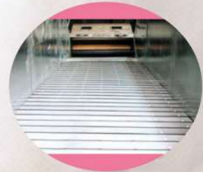
Internal view of lint slide for Humidification Humid Air Applicator
