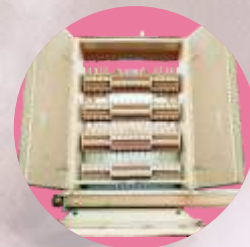
Trash Chamber with Roll, Jali & Screw Conveyor for Trash & Pink Boll worm removal
