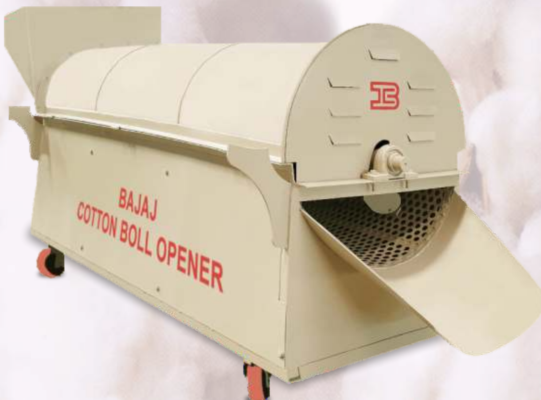
Easy to clean & maintain spiral screw Roll
