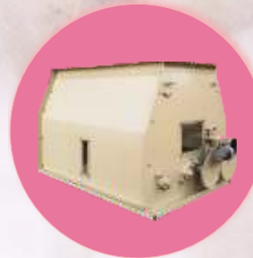
Twin Auto Regulator for Dividing Feed to Two Gin Machines
