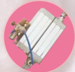
Pneumatic Cylinder with extra Air Reservoir for one time safe operation once change without supply of Pneumatic Air
