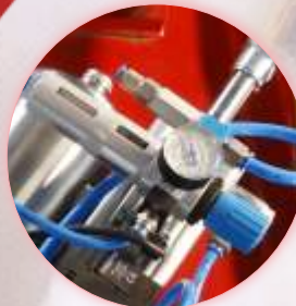
Inbuild with Heavy Duty Air Filter & Regulator
