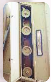
Taper Lock Pulley for Ease of Maintenance
