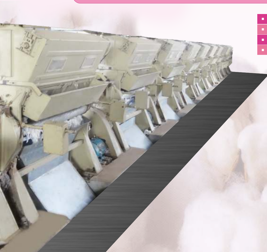
Intermittent Lint Suction Hopper With Pneumatic Valve
