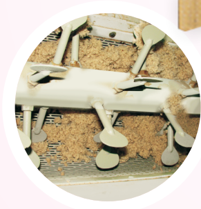
Bottom Beater Chamber for Pepper Dust Removal
