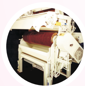
Easy Access for Saw Mandrel Inspection
